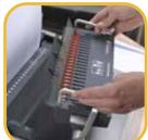
Satellite removable binding platform allows multiple users to punch & bind simultaneously reducing down time in the work place.
